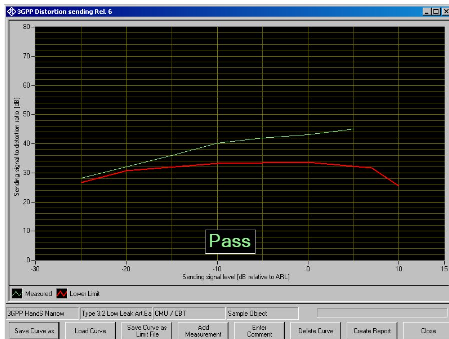
Fig. 38 Sending distortion measurement
